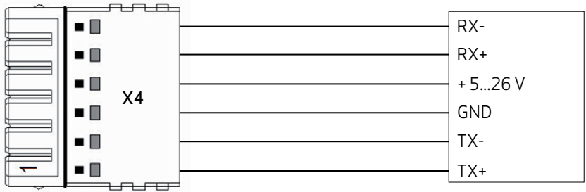
Fig. 9: Connector X4 pin assignment and external interface
